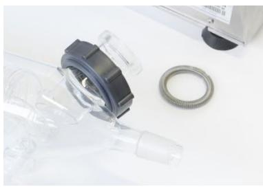
10. Mount the refrigerant fixing nut (6) in the refrigerant glass (3).
