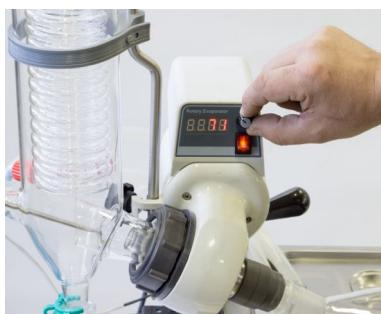
8. Turn the motor switch on (k) and adjust the speed with the knob (j).
