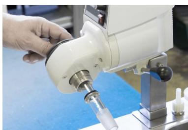
3. Install the flask connecting tube (12).
