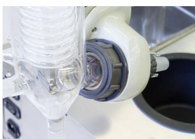
12. Fit the refrigerant assembly (3) in the angular reduction motor (10).
