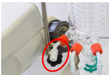
18. You must install the wide tube in the marked olive (in red). Cut before about two centimeters from the thin tube, as shown in the picture.
