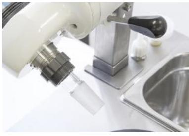
8. Install and tighten the flask fixing extension racord (13) of the sample.
