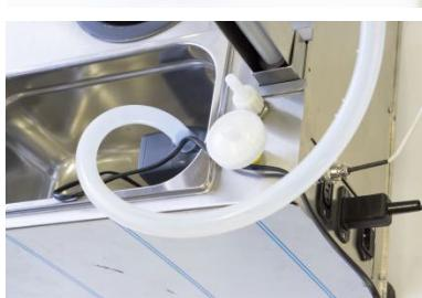
24. Install the refrigerant circulation pump (21) inside the cooling tray (19).
