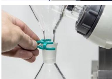
14. Install the receiving flask (9) with the clamp (4) by inserting it under pressure.
