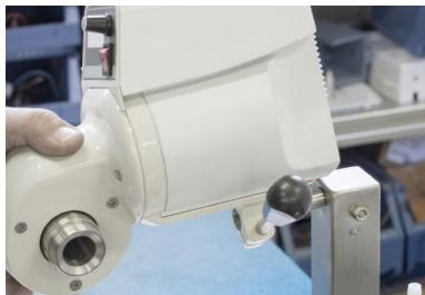
1. Install the angular gear motor (10) in its holder.
