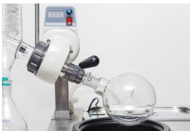
16. Instal the evaporator flask (14) with the flask fixing raccord (13).
