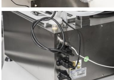
28. Detail of the connections from down to up: power outlet (18), coolant circulation pump (17) + (21), power connection reduction motor and temperature probe connection.
