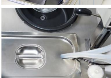
26. Once the refrigerant connection is completed, replace the lid to prevent loss of cold.
