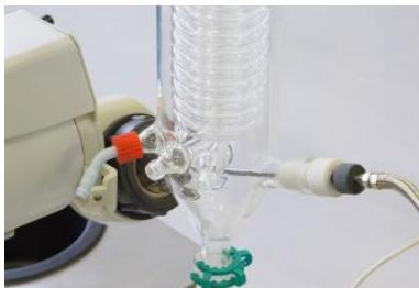
17. Install the olives and the inlet and outlet raccords (5) in the nozzles (22, 23, 24).
