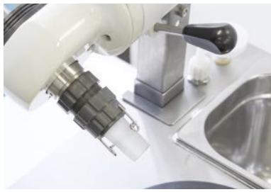
9. Install and tighten the flask fixing racord (13) of the sample.
