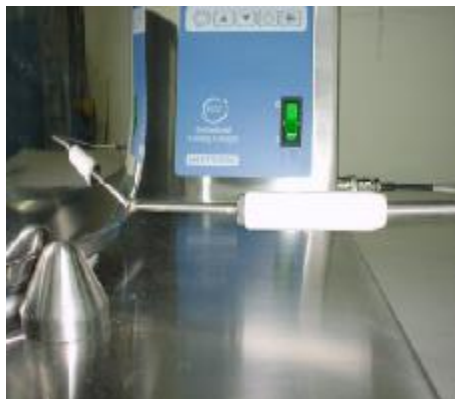
Pic 7. probe placed in the housing at the base of the pot
